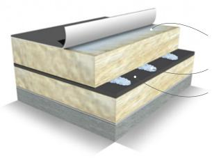
Bonding fleece-backed synthetic roofing membrane to insulation.
