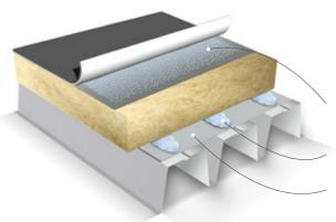
Bonding fleece-backed synthetic roofing membrane to insulation.
