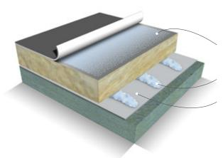
Bonding fleece-backed synthetic roofing membrane to insulation.
